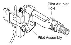
Figure 44 - Pilot Inlet Air Hole
